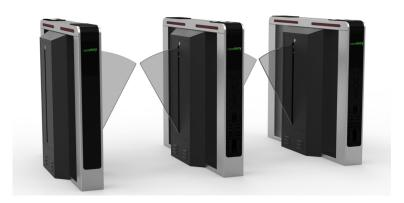
The Nexakey NX-FBL2520 is a high-performance flap barrier gate with a sleek SUS304 stainless steel body, designed for secure and efficient pedestrian access. With a 550 mm passage width and durable 24 V DC brushless motor, it ensures smooth, quiet operation. Infrared sensors prevent tailgating, and in emergencies or power failure the barrier opens automatically to allow safe exit. Ideal for office lobbies, banks, hospitals and other high-traffic indoor spaces.
